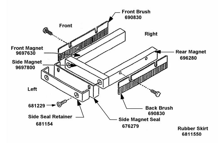
This magnet and seal illustration shows how the machine is set during the right side edging mode. This is achieved by simply removing the right side retainer, right side magnet seal and the right side magnet. For normal (non-edging) operation, the right and left side arrangements are identical. For left hand edging, reverse the above arrangement from right to left.
